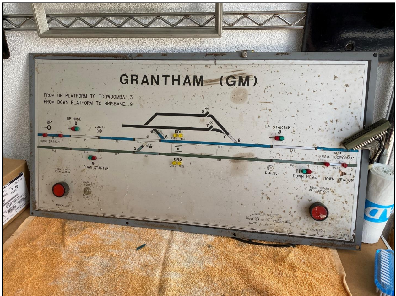
Above: Removed from the metal frame and partly cleaned to remove dust and bird droppings, more cleaning was required to try and remove other marks and stains.
