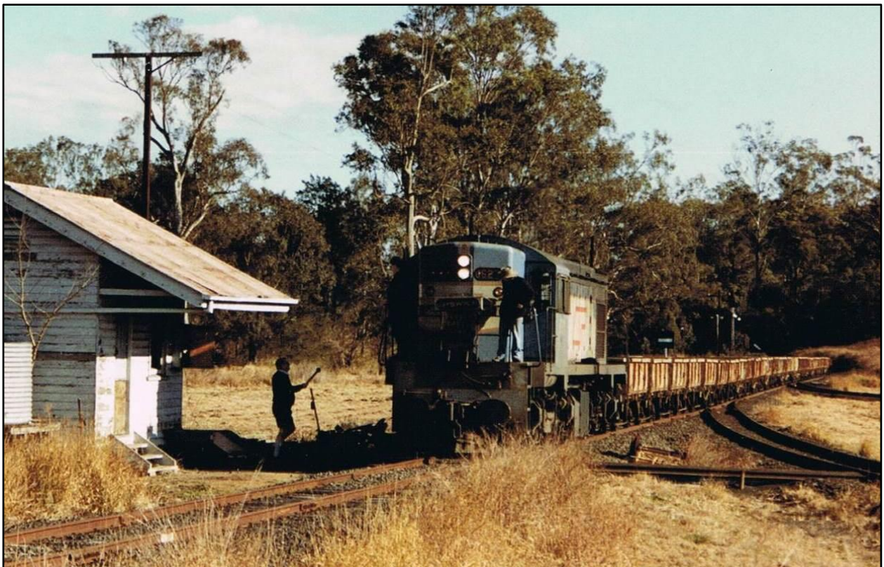
Above: An empty spoil train pauses at Box Flat in 1989 to change the Ordinary Staff before proceeding onwards to Swanbank. The trailable facing points indicator (in reverse) can be seen above the wagons and the Up Home signal at 'proceed' is at the rear of the train.
